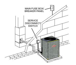
NOTE—Units are approved for use only with copper conductors. Ground unit at disconnect switch or connect to an earth ground.
